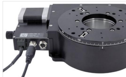
Devices connect to a 24-48VDC power supply. The number of devices you can power will depend on the combined draw of the devices and the current capacity of the power supply.
