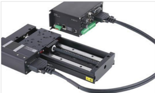
Depending on the controller and peripheral, the motor cable may be an MC03 (DB-15 M-F), MC10T3 (DB15 to DB26), or MC10 (DB26 M-F) cable. Cables are high-flex with specific wire bundling; using cables from Zaber is recommended.
